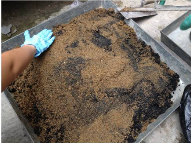
Figure 4. Real sediments sample from Tsuen Wan box-culvert near exit
